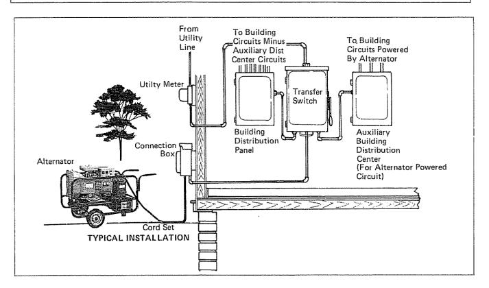
A typical Stand-By Power System is shown above. This System uses a (1) Connection Box and Cord Set, (2) a Transfer Switch, (3) two Building Distribution Centers, and (4) interconnecting wiring.
